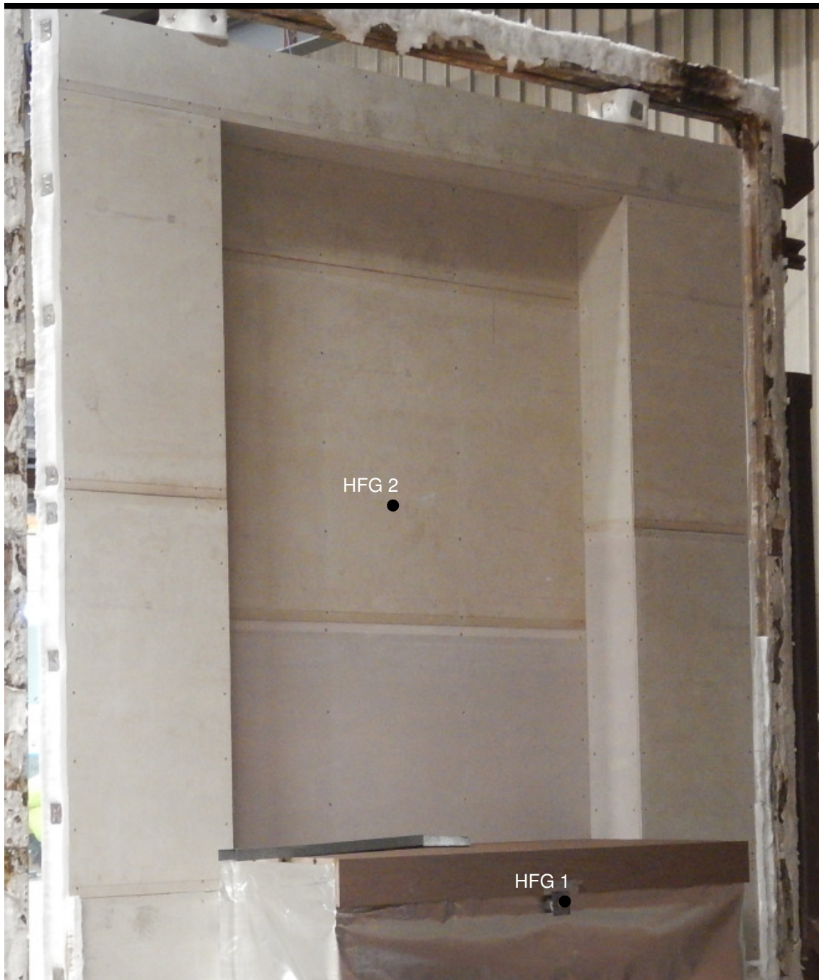
Figure 4 Indicative heat flux gauge locations (exposed face)
