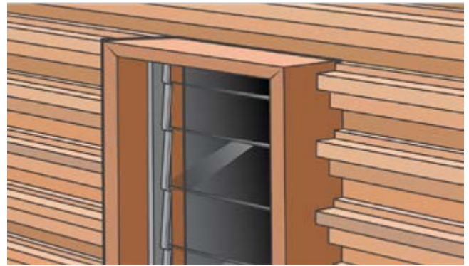
Figure 6: Bold and prominent window stop that frames the window. Window stop is DAR 140 x 30mm. Wall is clad in Castelation® Stepped Expression combination.
