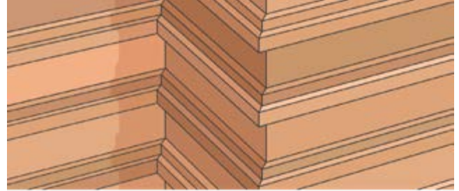
Figure 5: Mitred corners shown on Castelation® Stepped Combination. Modinex recommends using external glue on all mitre cut corners to resist the corners opening up over time.
